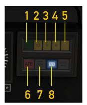
Apart from the DVD lamp that we have already encountered above, in this panel we find eight lamps that alone or in combination can display the different states that the ATB can assume. When ATB is not active, lamp 8 (BD = out of service) lights up. Lamp 7 (brake contact) is shown when the Mc applies the train brakes — even when the ATB is switched off.
