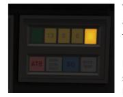
We will now explain the operation of the activated ATB by means of an example. In the left image we are driving at a speed of 125 km/h. Then, in the right picture, a 40 km/h speed limit has been detected. A bell sound ('ting') can be heard and lamp 5 lights up.
