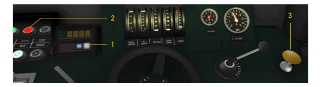
This system expects the Mc to click the vigilance button (3) or press the numeric ENTER key at least once every half minute. When 30 seconds pass without any of these actions, a buzzer will sound and a flashing red light (2) will appear on the steering table. From that moment on, the Mc has five seconds to respond. Failing this, the DVD will trigger an emergency brake action. Controls will be locked until after the train has come to a complete stop.
