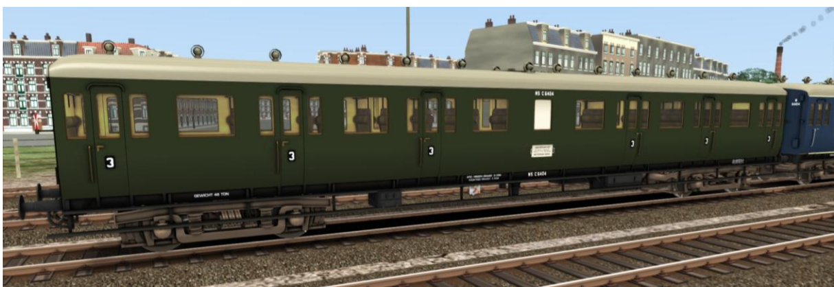
Steel compartment carriages C12c Series C 6400
